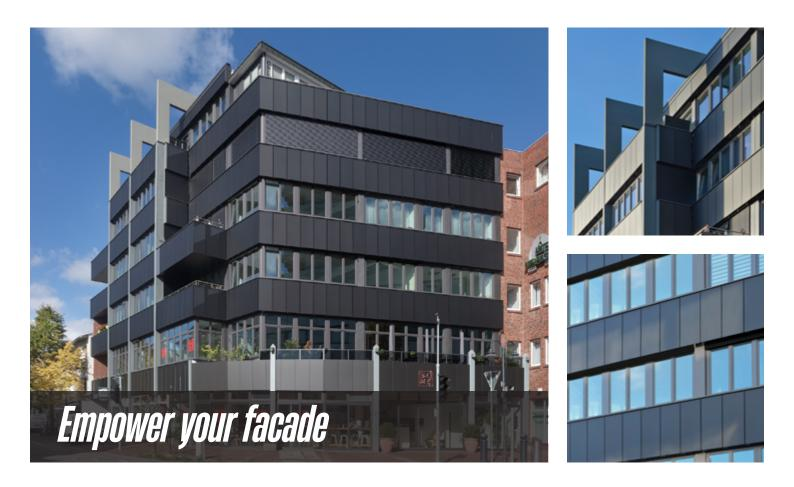
50-year-old building was completely renovated, technically and energetically brought up to date according to Energy Efficiency 100. 234 anthracite-colored SKALA modules were integrated into the facade below the window strips and on the parapets.
